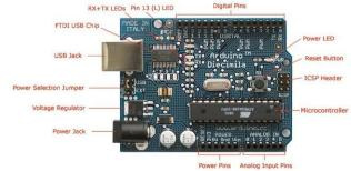
Fig. 1 Arduino embedded board with microcontroller
